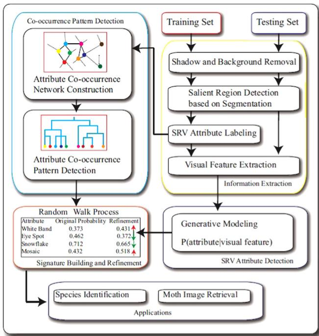
**Fig. 4.** The flowchart of the proposed moth species identification and retrieval system. It consists of (1) information extraction, (2) SRV attribute detection, (3) attribute co-occurrence pattern detection, (4) signature building and refinement, and (5) moth identification and retrieval applications.
